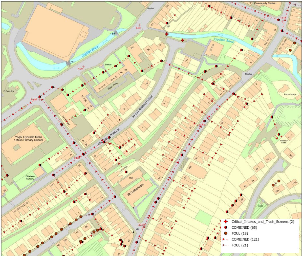
Figure 8 – Map of DCWW foul and combined sewer assets at St Catherine's Close.
