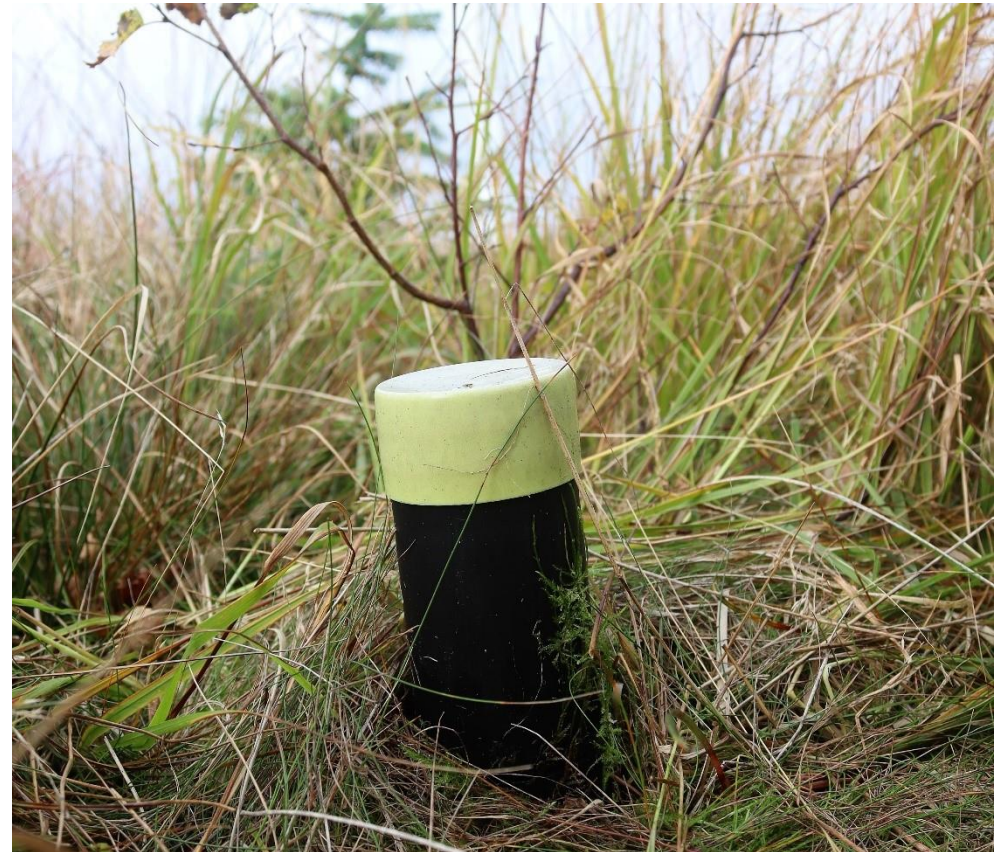
Figure 7: Peatland 'dipwell' housing an automatic water level reader. Image: LPSW
