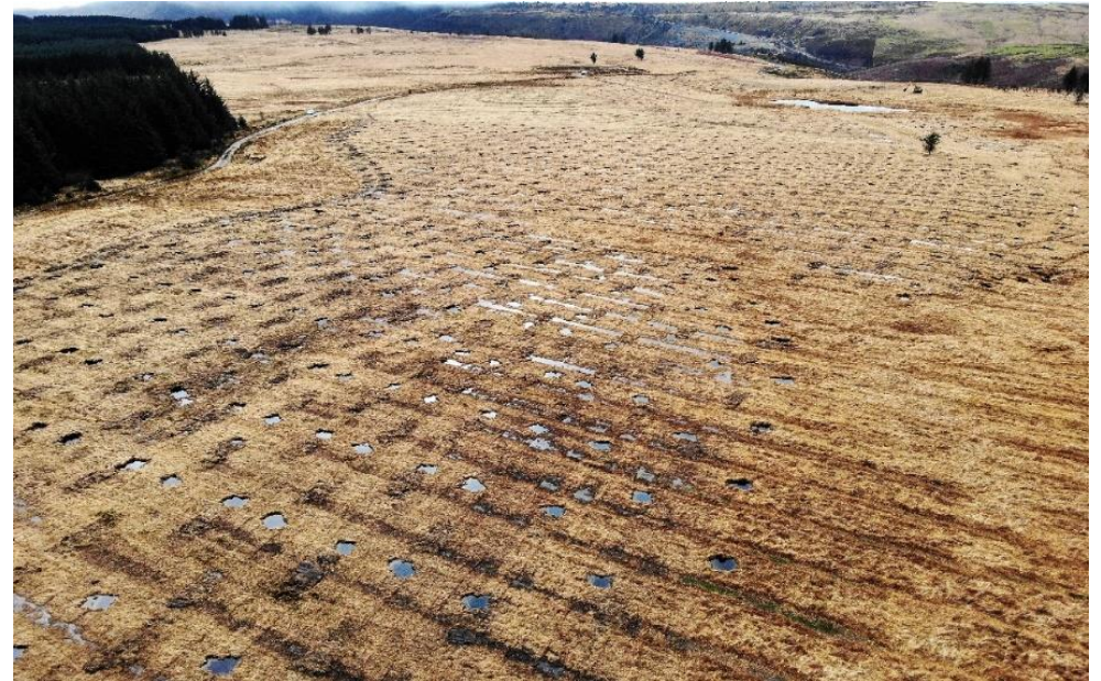
Figure 1: Castell Nos HRA - aerial shows blocked plough lines and 'borrow pits' where peat has been extracted and used for dams. Image: LPSW
