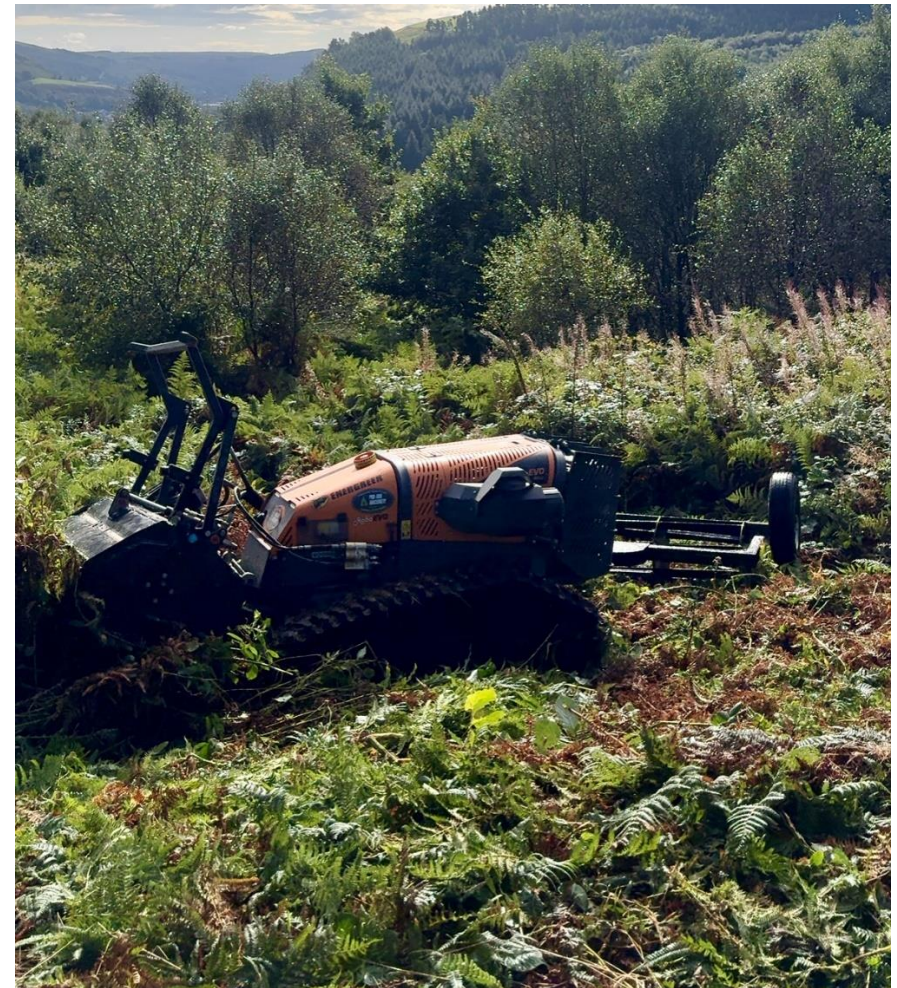
Figure 15: Cwmparc CWS - bracken control with robo-flail and roller. image: LPSW
